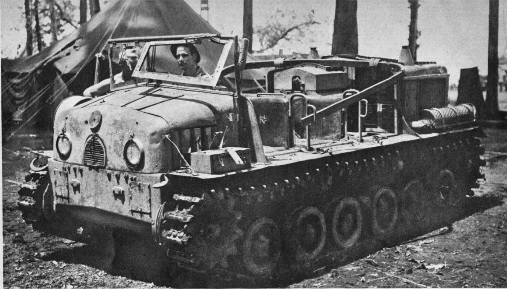
SIX-TON PRIME MOVER, TYPE 98 (1938) IS USED BY JAP ARMY TO TOW HEAVY ARTILLERY, CARRY AMMUNITION. IT DOUBLES IN RECONNAISSANCE DUTY
